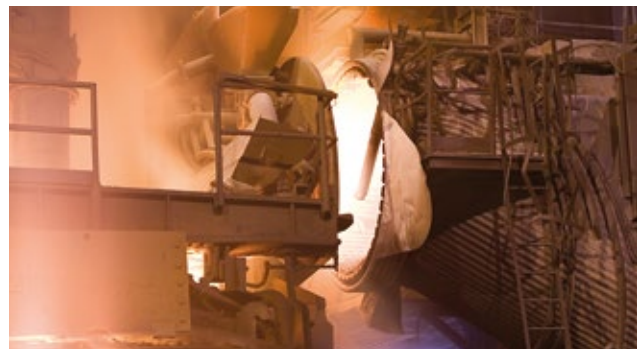
The off-gas analyser probe location of the EFSOP® NextGen system on the fume duct
