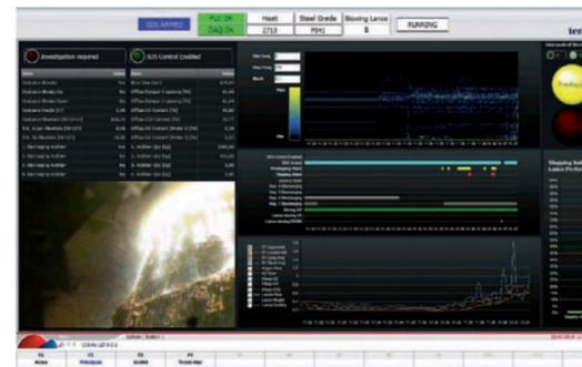
iBOF® Intelligent Slopping Detection System main screen.
