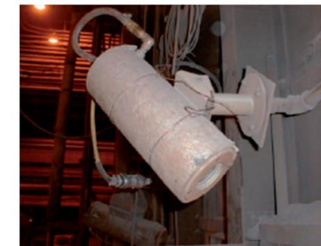
Typical installation of the iBOF® tapping camera.
